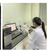
UV-visible Spectrophotometer GENESYS 10S UV-Vis model (Thermo Scientific) is an analytical instrument used in study program and research activity in the Faculty of Pharmacy, University of Puthisastra. This machine has a wavelength range from 190 nm to 1100 nm. It is easy to use to demonstrate or evaluate the accuracy of a test for correctly identifying some condition.
