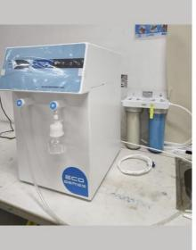
The faculty of Pharmacy has ordered a new water purifier that will provide a lot of ease of use in the faculty, especially the purified water that is suitable for use with the HPLC machine, which requires the use of well-purified water. This Eco water purification system ensure high quality ultrapure water, in addition to reverse osmosis water.
